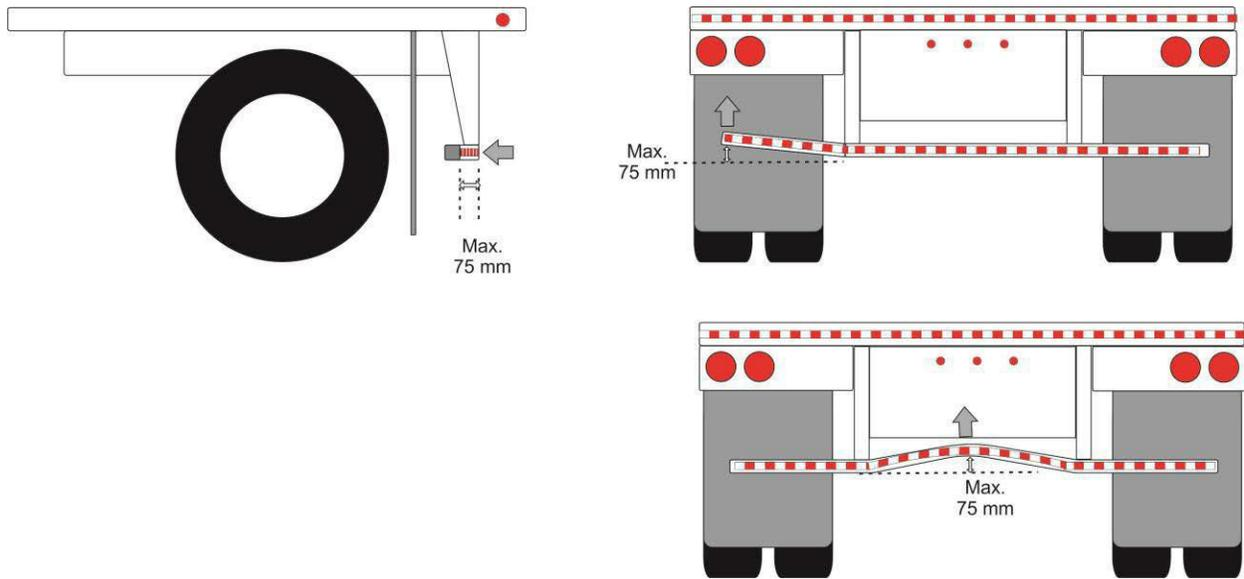
Figure 3 – Example of Damaged Vertical RIG member
