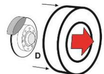
E. Limited-inspection of disc brake (this is an inspection of visually accessible components and measurement of the friction material of one brake pad)
